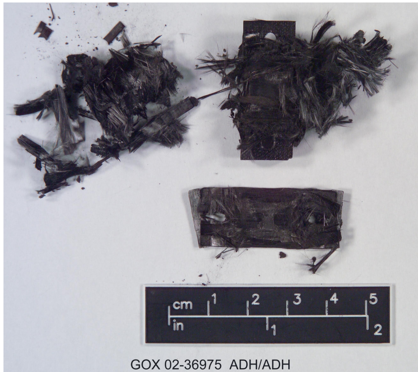
FIG. 5— Posttest sample for FM 57 (Adh/Adh) (typical for all GOX ignition results).
