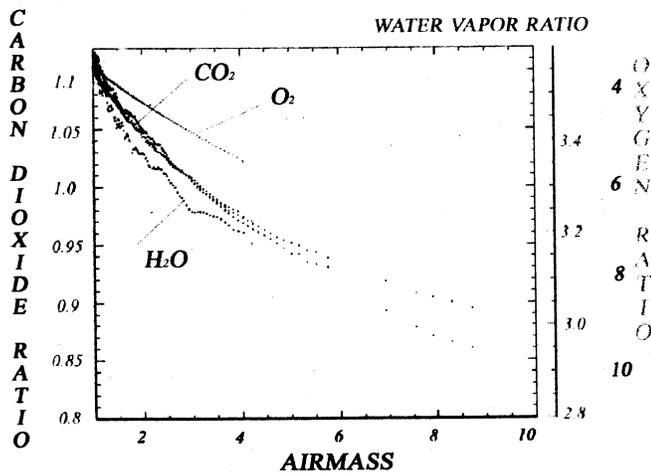
Fig. 4. Here the ratios from the previous figure are plotted against the calculated air mass. The AM and PM values for O<sub>2</sub> are virtually the same and cannot be distinguished. The CO<sub>2</sub> channel shows some slight variation throughout the day probably arising from consumption by plants. The water vapor channel shows considerable variation consistent with typical changes in humidity throughout a day.
