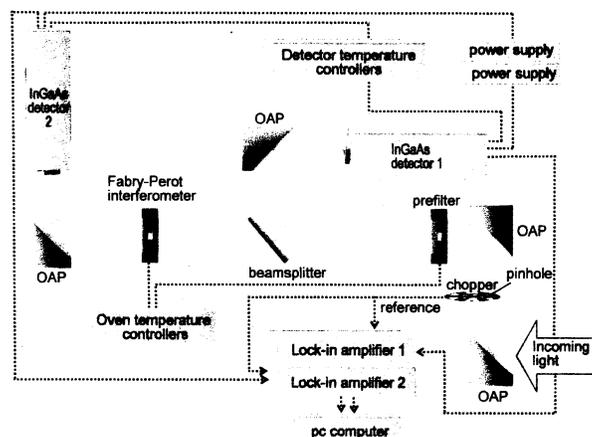
Fig. 1. Optical and electronic schematic for the CO<sub>2</sub> channel of the Fabry-Perot instrument. Incoming light is collimated by two off axis parabolic gold mirrors (OAP's). The light is divided into Fabry-Perot (detector 2) and reference (detector 1) sub-channels, measuring changes in CO<sub>2</sub> absorption and solar flux, respectively. The ratio of these signals can then be related to changes in the CO<sub>2</sub> column.
