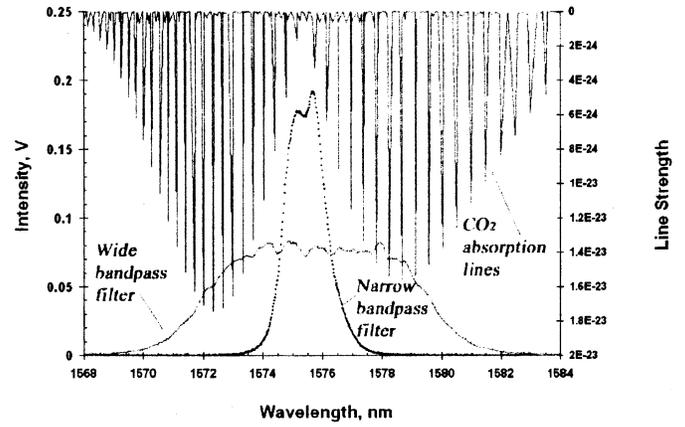
Fig. 8. Laser scan of the two filters for the small CO<sub>2</sub> radiometer. The CO<sub>2</sub> absorption lines from HITRAN database are also shown. The narrow band versus wide band sub-channels ratio will be sensitive to CO<sub>2</sub> changes in the atmosphere.
