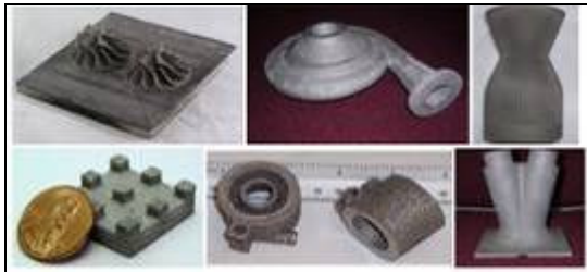
Figure 9. Titanium Parts Produced by EBM Process
