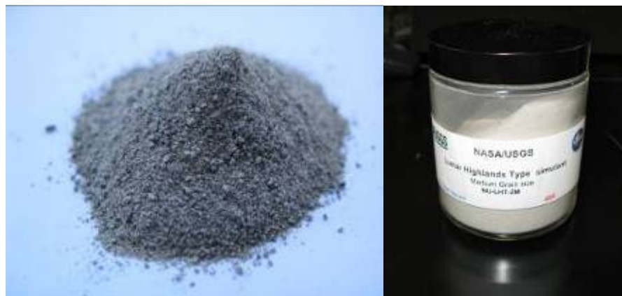
Figure 5. NU-LHT-1M and Jar of NU-LHT-2M Simulants
