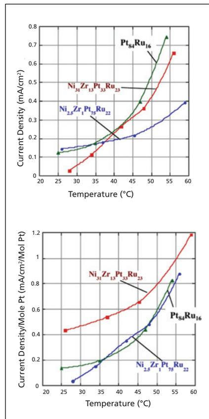
**Plotted Test Results** compare current densities for Pt<sub>33</sub>Ru<sub>23</sub>Ni<sub>30</sub>Zr<sub>13</sub> with current densities of the state-of-art Pt-Ru under the same test conditions.
