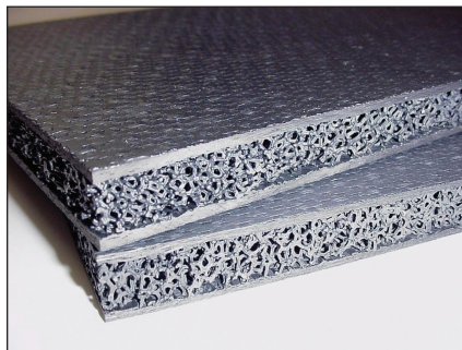
The Foam Core Ceramic Matrix Composite is a weave SiC and carbon fiber, which allows heat dissipation in-plane. Face sheet thickness is nominally 2.4 mm, and core thickness is 1.26 cm.
