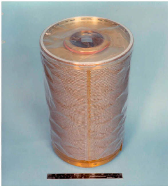
Figure 2. US LiOH canister on ISS and Shuttles.
