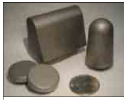
Figure 1. Examples of UHTC Components are shown that have been tested in the NASA Ames Arc Jet facility to evaluate the materials response in a simulated reentry environment. The cone and wedge models are representative of the scale and geometries anticipated for use on UHTC sharp leading-edge vehicles.
