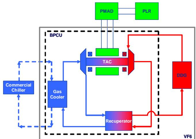
Figure 3.—DDG/BPCU test schematic.
