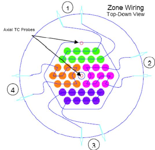
Figure 4.—DDG electrical wiring zones.
