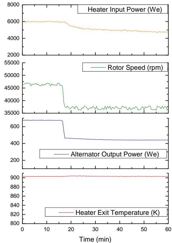
Figure 9.—System response using DDG PID HET control.
