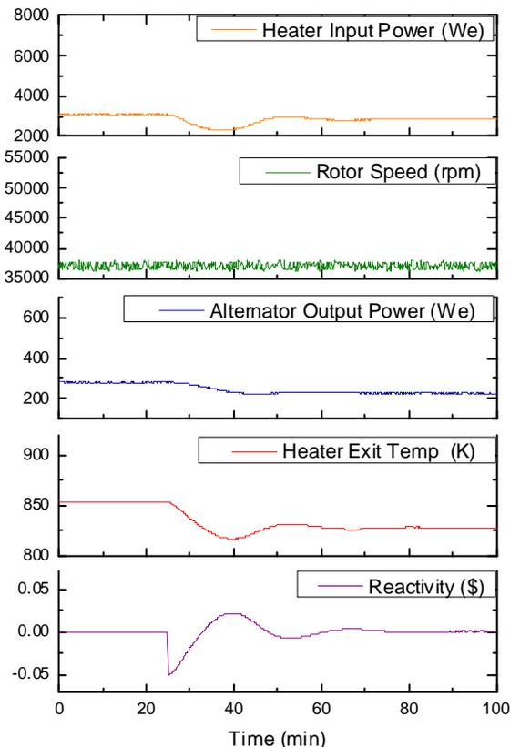
Figure 11.—DDG simulated reactivity response to a step change in shaft speed.
