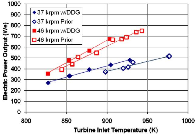
Figure 7.—DDG-BPCU test steady-state power output comparison.
