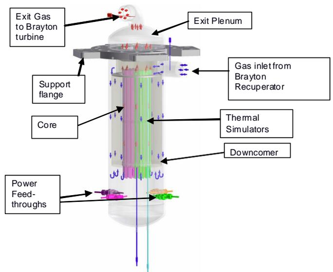
Figure 5.—DDG flow path.
