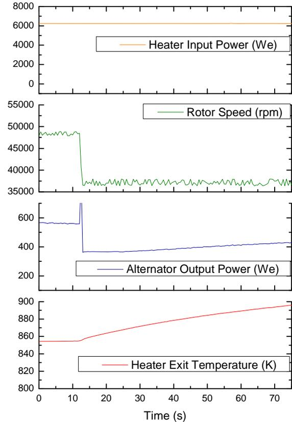
Figure 8.—System response at constant DDG power.
