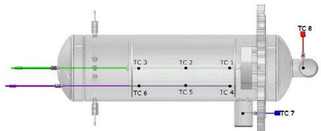
Figure 6.—Schematic of DDG thermocouple placement.
