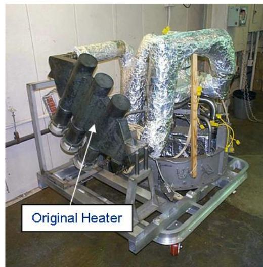
Figure 2.—Previous BPCU gas heater (shown uninsulated).
