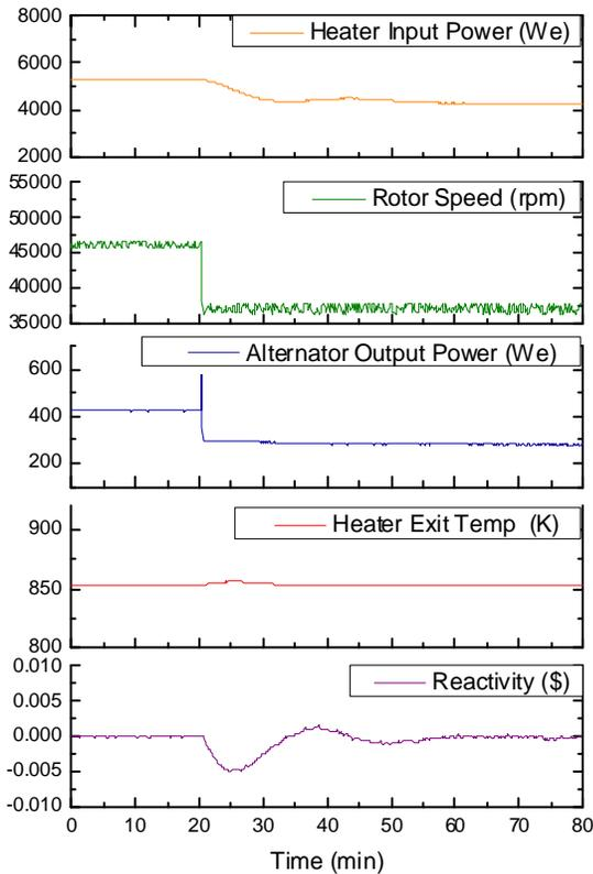
Figure 10.—System response using simulated DDG reactivity control.
