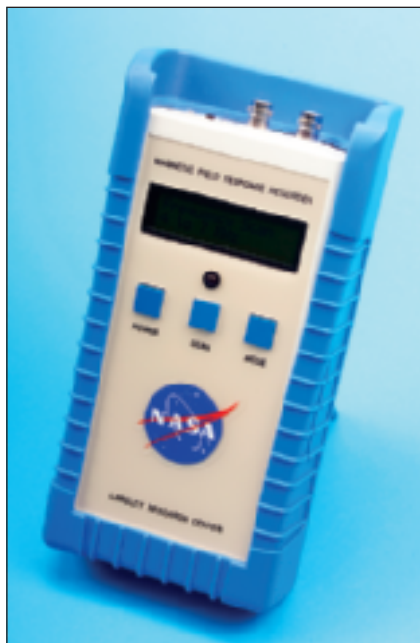
Figure 1. A Portable Magnetic-Field-Response Recorder is shown in a handheld version.
