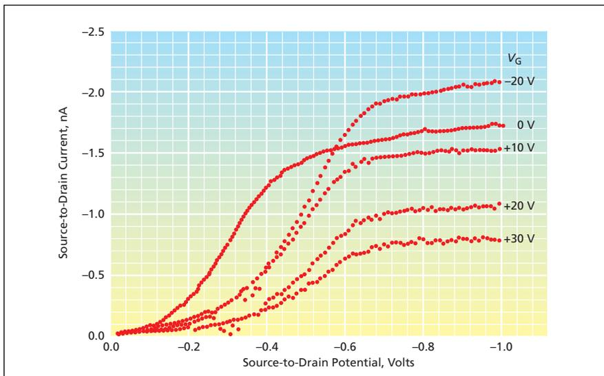
Figure 2. These **Current-Versus-Voltage Characteristics** were obtained from measurements on the FET of Figure 1. The measurements were made at various values of back gate voltage ( $V_G$ ) representative of the accumulation and depletion modes.
