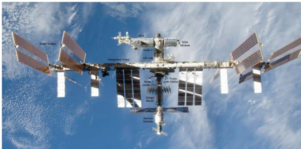
Figure 4. International Space Station, Present Configuration
