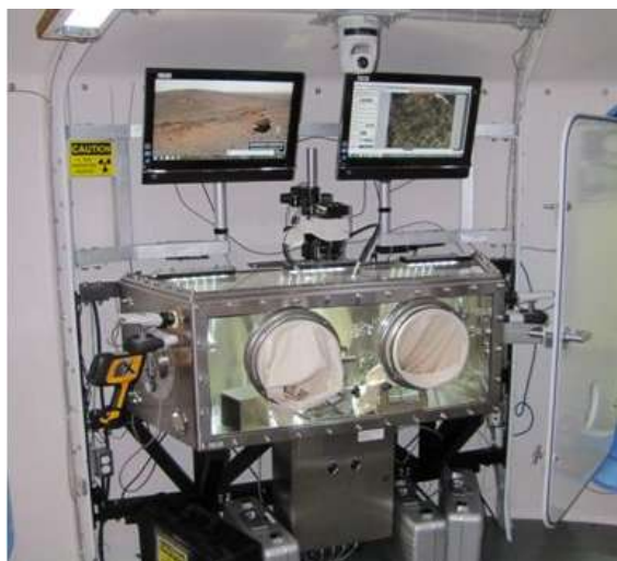
Figure 1: GeoLab integrated into the HDU1-PEM. The suite of instruments included a handheld XRF analyzer (far left), stereo microscope (center, above glovebox), network cameras, and touchscreen computers. Ports in the back of the Glovebox are pass-through chambers for sample transfer from the outside.
