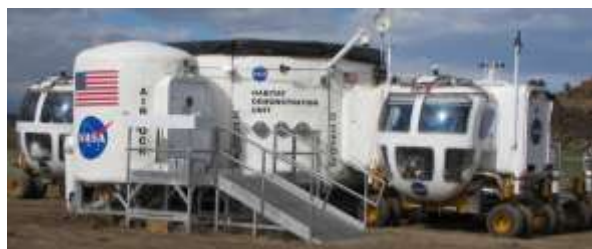
Figure 2: The HDU1-PEM with two rovers docked. The three circular ports directly below "Habitat Demonstration Unit" are the antechamber doors that provide access directly into the GeoLab Glovebox.
