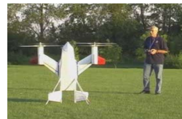
Figure 13. Puffin 1/3 scale flight demonstrator.
