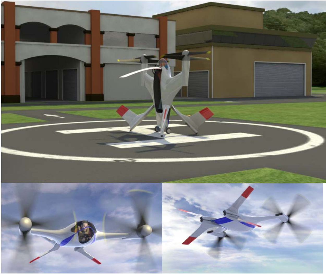
Figure 3. Features of the NASA Puffin electric VTOL concept. Top shows the vehicle with the takeoff and landing gear articulated outward for improved tip-over characteristics. Bottom shows the vehicle in flight as a minimal wetted area design solution for high cruise efficiency.
