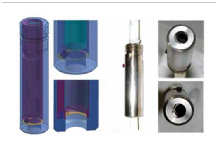
The Rolling-Tooth Design of the core breakoff and retention mechanism (left), and the assembled parts (right).
