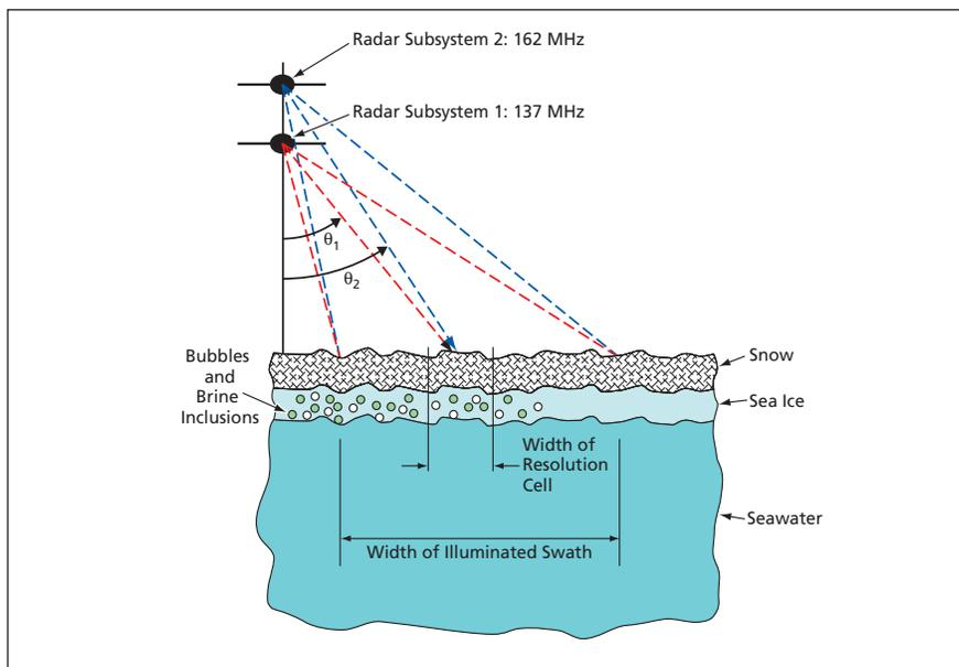
**Two Chirped VHF Radar Subsystems** operating about different nominal middle frequencies targets the same surface area from two slightly different angles. Frequency- and spatial-domain interferometric computations performed on the radar backscatter signals enable determination of the thickness of the sea ice.
