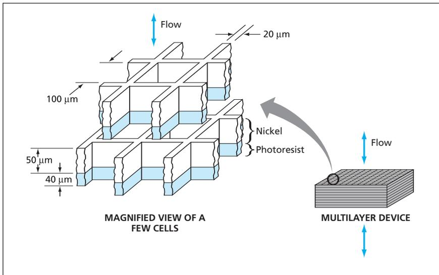
Figure 1. The Configuration of This Device Is Typical of a microscale heat exchanger as described in the text. The materials and dimensions shown here are representative rather than exclusive: they were chosen in a design trade study in which account was taken of capabilities for fabrication and of requirements for low axial thermal conduction and low pressure drop under a specific set of assumptions.
