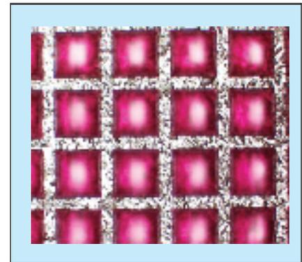
Figure 2. A Microphotograph of a portion of one layer of the fabricated microscale heat exchanger shows the grating structure and surface features of the nickel sublayer.
