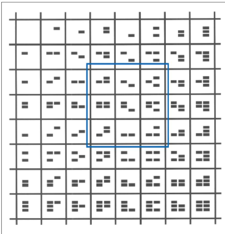
Figure 2. In the **Coded Cartesian Grid**, each grid cell contains a distinct binary image code that identifies that cell. The upper code bits in a cell identify the line at the bottom of the cell, while the lower bits identify the line at the left of the cell. In the instantaneous field of regard (square box), code bits identify vertical lines 2, 3, and 4, and horizontal lines 3, 4, and 5.
