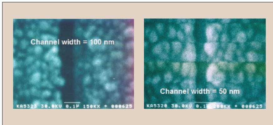
These **Scanning Electron Micrographs** show channels of two different widths that were fabricated by the present method. In a finished device, the channels would be covered with an SiO<sub>2</sub> membrane, which would be sufficiently transparent to enable analysis of specimens in the channels by use of a fluorescence microscope.
