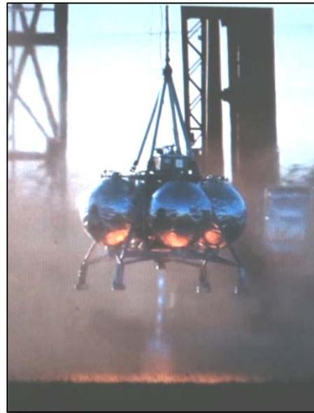
Despite the vertical oscillation, the test was proceeding towards its full hover duration until a load cell data cable snagged on the top of the vehicle, causing a pitching moment that resulted in a attitude rate limit violation that triggered the on-board soft abort logic. The vehicle slowly descended until the landing indication resulted in engine shutdown after a total run time of 20 seconds instead of the intended 30 seconds.
