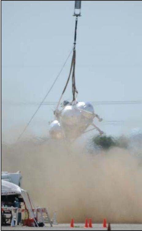
This uncontrolled motion continued despite on-board software and ground commands for soft and hard abort engine shutdown. These primary methods for engine shutdown all rely on the throttle valve, which had failed to full open. After 13 seconds of erratic flight the thrust was finally terminated when the wired FTS system was manually activated. Since the vehicle was tethered to the crane, no vehicle damage resulted from this test.
