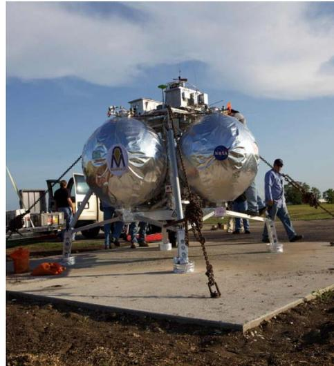
This test was also designed to verify the second FTS radio frequency operating in the VHF band. All previous tests had used one UHF radio signal to close both the LOX and LNG thrust termination valves. Adding a second independent radio and frequency provides the redundancy needed to allow free-flights at JSC, since closing either the LOX supply (via one radio) or the LNG supply (via the other radio) will terminate thrust.
