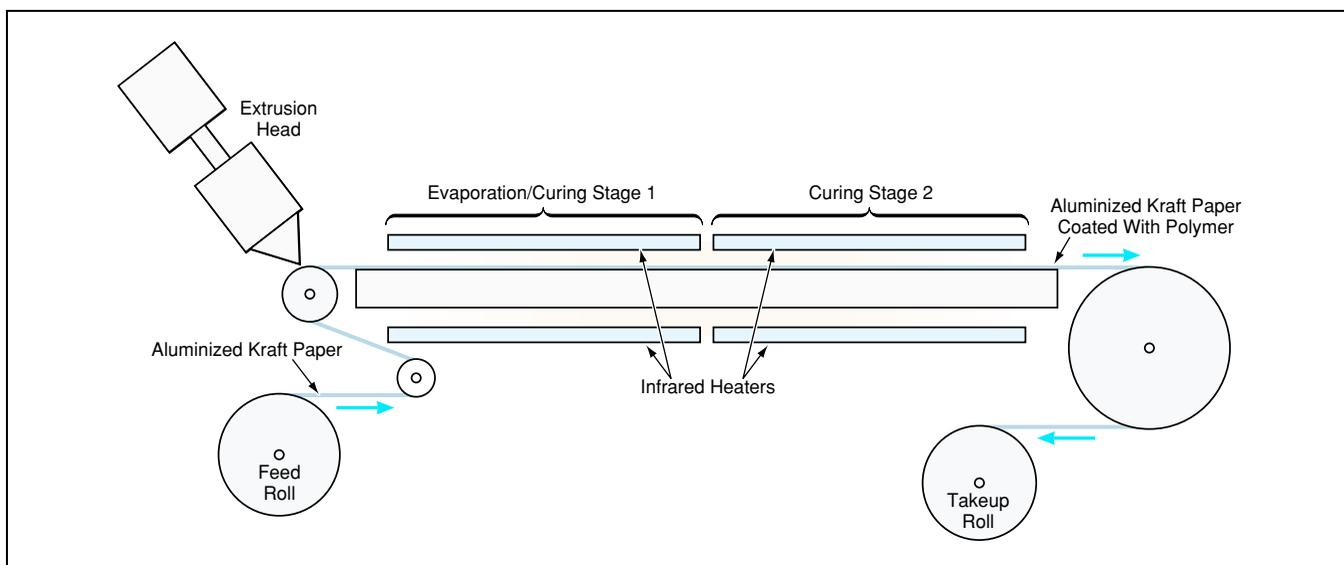
**A Film of Dielectric Polymer Is Cast** on a continuous strip of aluminized kraft paper. High dielectric performance is obtained through selection of the materials and design of the process and machinery.
