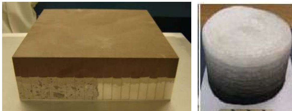
Advanced rigid TPS materials with functionally graded material composition.
