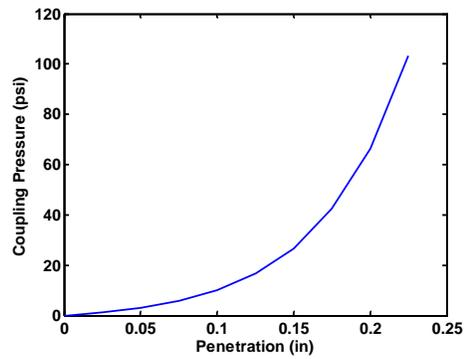
Figure - Fluid Structure Interaction (FSI) Coupling Curve
