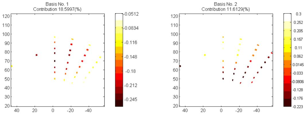
Figure 11. Contour for first two pressure basis vector using 33 measured locations
