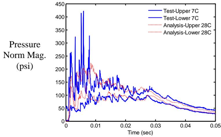
Figure 5. Pressure data uncertainty bounds for T300-30 (solid-blue) using 7 tests and uncertainty bounds for analysis (dashed-red) using 28 cases
