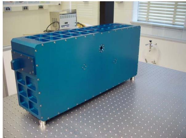
Figure 5: First version of a compact-packaged, coherent lidar transceiver. The transceiver comprises the pulsed 0.25-J, 10-Hz laser, CW seed laser, lidar transmit-receive switch, and dual-balanced detectors. The beam exits from the side hole.
