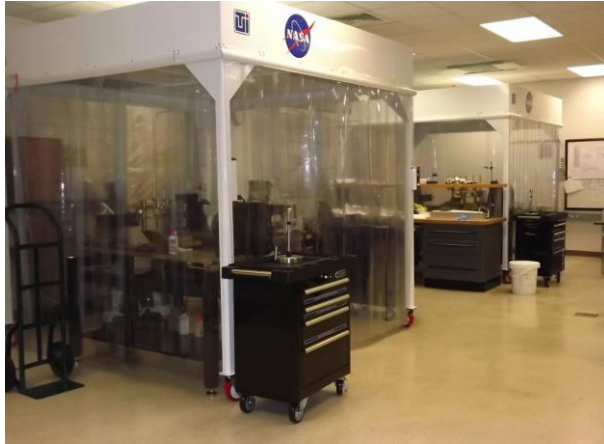
Figure 4. ART polishing stations under clean room tents in the mandrel production area.
