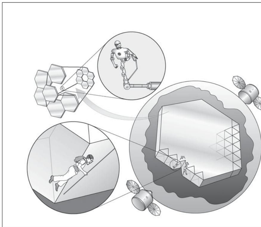
An artist's rendering of the **Shirtsleeves Assembly Hangar**. At the lower right is a cutaway of the inflated fabric sphere that houses astronauts in oxygen masks and backpacks. The humans would work with a robot to accomplish the final telescope assembly.
