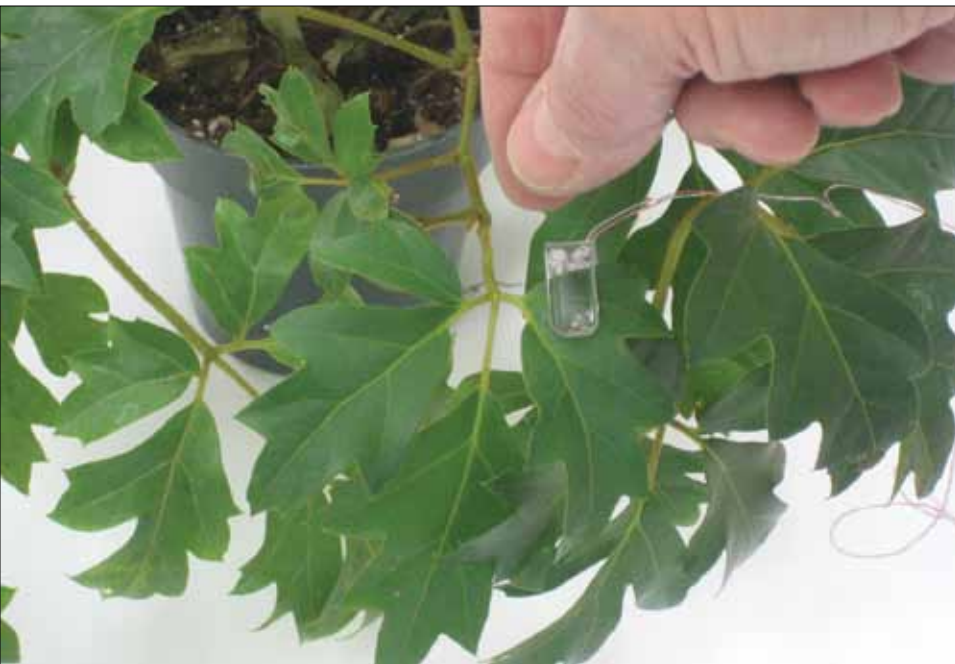
By measuring electrical pulses, AgriHouse's sensors can determine several characteristics important to plant health. The sensors can remain attached through wind and rain while leaving the plant unharmed.
