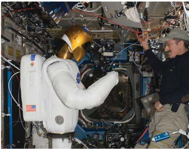
Figure 9: Robonaut - Robotic Assistant Payload Onboard ISS
