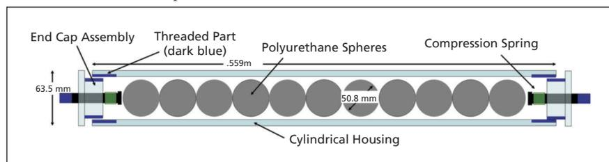
Figure 1. Initial schematic for the **Vibration Suppressor**. Pistons at each end of the cylinder make contact with the granular chain of spheres. Static compression of the granular chain is achieved through the use of soft springs located between the pistons and end caps, which screw onto the container.
