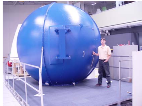
Figure 2. The Holodeck. The double-hinge-style door is visible, as is its magnitude and composition. Technically considered a confined space until the ventilation system is installed, it has the capacity to fit two or three adults comfortably. The floor is modular, and the whole dome has been placed on an 80/20-style raised floor and added supports.
