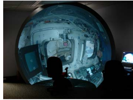
Figure 1. The iDome. Paul Bourke’s standing hemispherical system, using a single projector for gaming and education visualizations.
