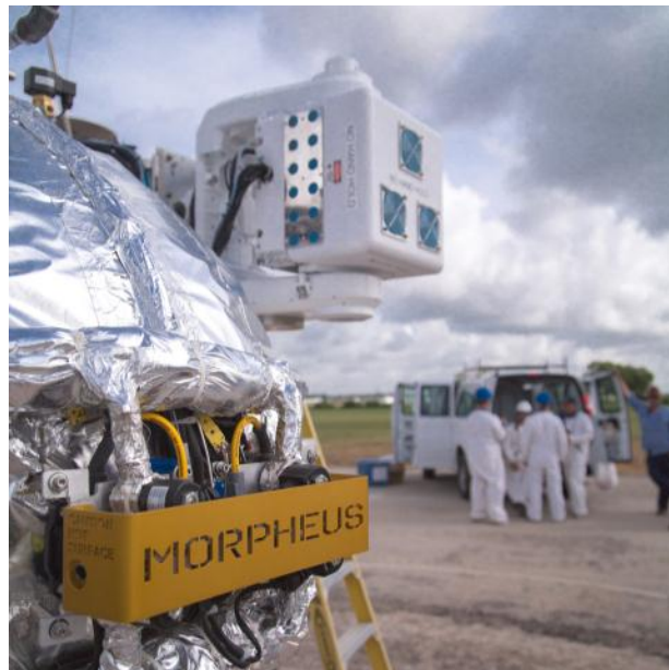
Figure 2 – ALHAT Hazard Detection System mounted on the Morpheus 'Bravo' vehicle
