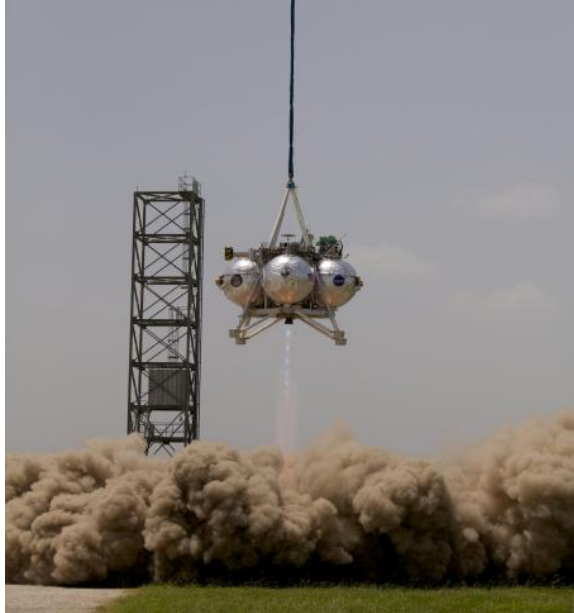
Figure 10 – Morpheus 1.5 'Bravo' executing a translational Tether Test in August 2013. Mars soil simulant was deployed on the launch pad to study plume impingement for the Mars 2020 program.
