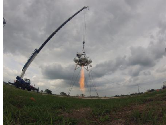
Figure 5 – Morpheus in standard Hot-fire Test Configuration
