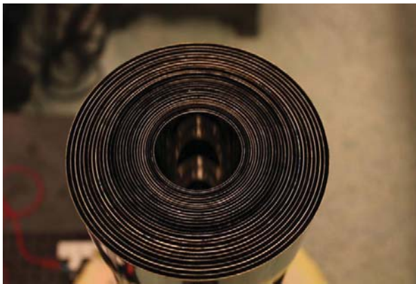
Figure 7. 28 mirror shells installed into the ART-XC flight module
