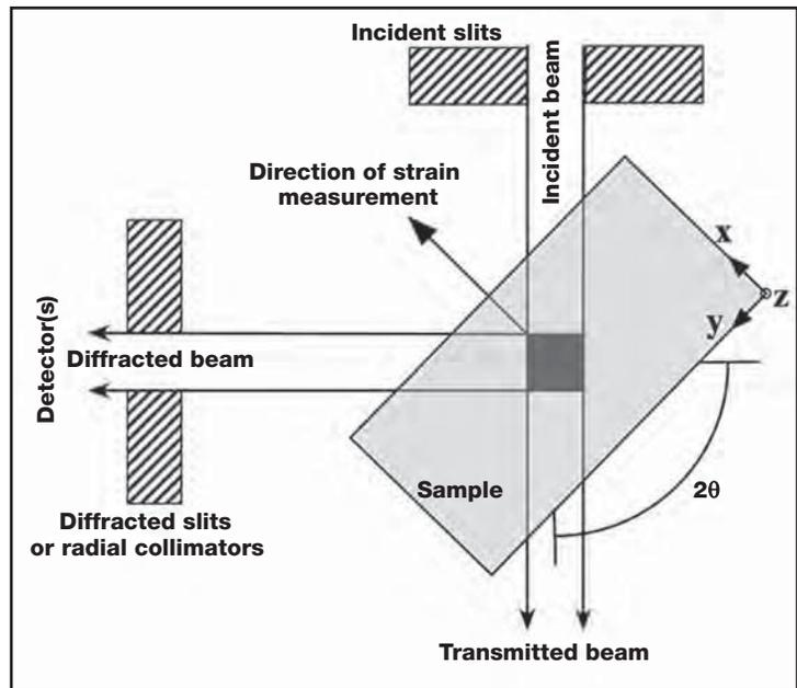
Fig. 4 — Schematic of neutron diffraction set up viewed from above shows nominal gauge volume (dark square) as defined by the slits<sup>[7]</sup>.
