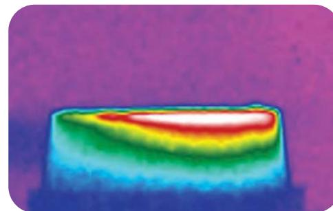
**Fig. 2** — Thermal image of a layered additive manufacturing process shows significant temperature gradients near the deposition zone<sup>[1]</sup>.
