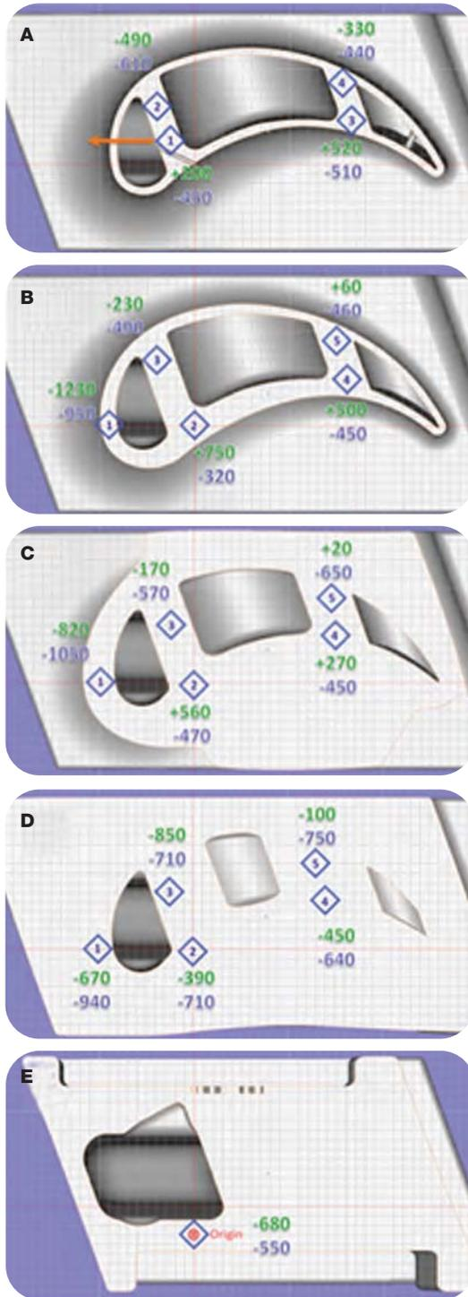
compressive and much more uniform throughout the lower portion of the blade, suggesting that the blade will be less likely to distort during service. The combination of neutron tomography and residual strain measurement is a critical approach for examining complicated components that can be built using additive manufacturing.
