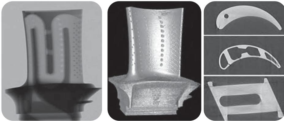
**Fig. 3** — Neutron radiograph (left), volume rendered (center), and transverse slices at top, middle, and bottom (right) of turbine blade fabricated using additive manufacturing. Blade height is ~76 mm.
