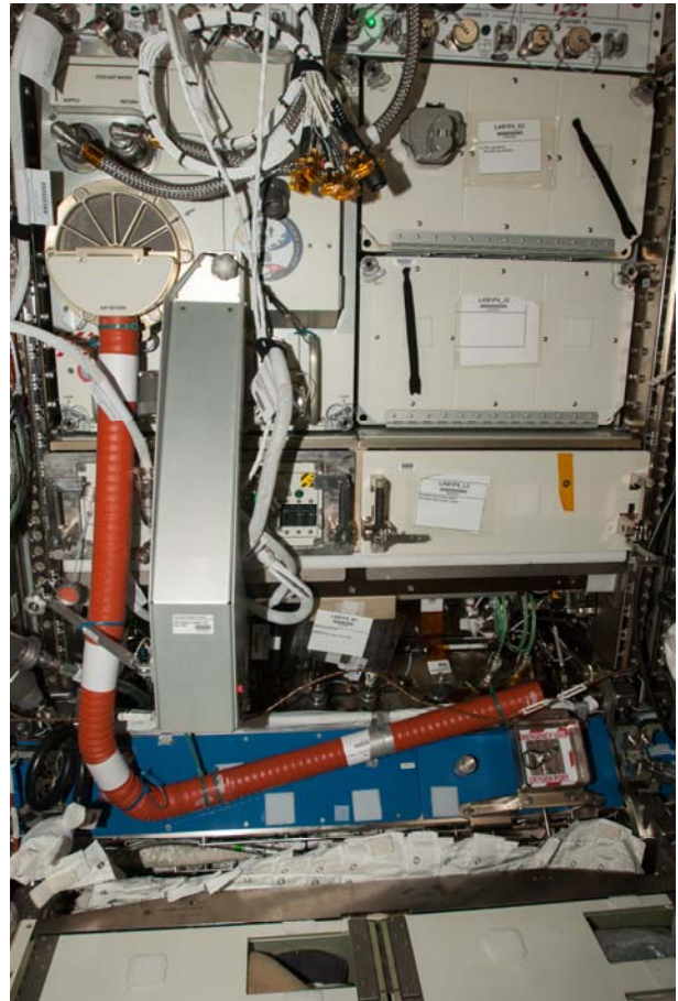
Figure 4. Amine Swingbed Payload installed in EXPRESS rack 8, in the LAB1P4 location.
