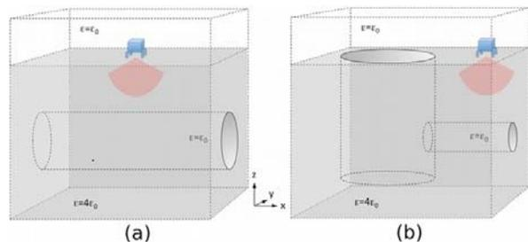
**Figure 1 (bottom left column):** Idealized scenarios for simulating GPR returns near a lunar pit. (a) Rover investigates an underground lunar tunnel. (b) Rover investigates a tunnel attached to a lunar pit.
