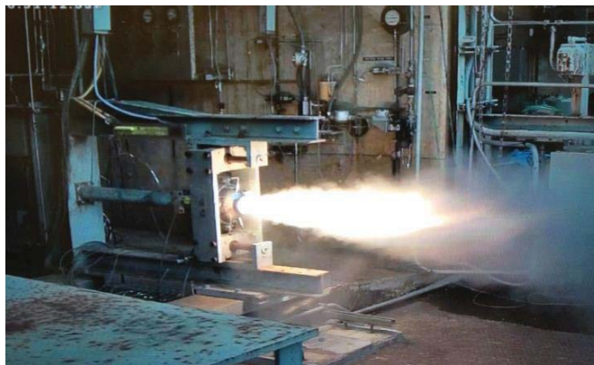
Figure 3. Static test firing of the first “printed” titanium solid rocket motor case.
