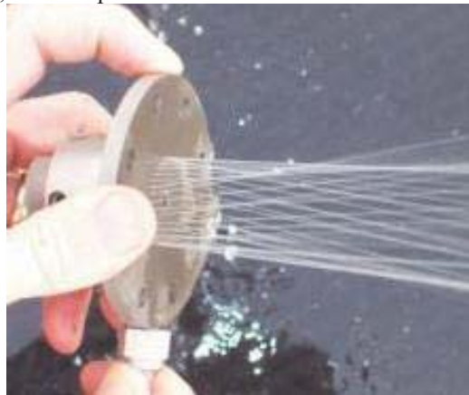
Figure 8, Fuel film cooling circuit for a liquid oxygen/propane injector.
