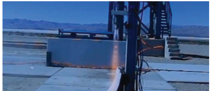
Figure 5. The University of California, San Diego liquid oxygen/RP additively manufactured engine static test firing.
