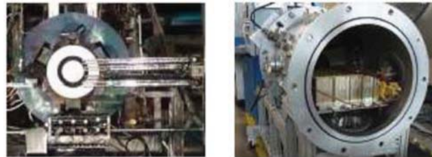
Figure 6 HIVHAC EDU Thruster and Colorado Power SBIR PPU undergoing performance testing.
