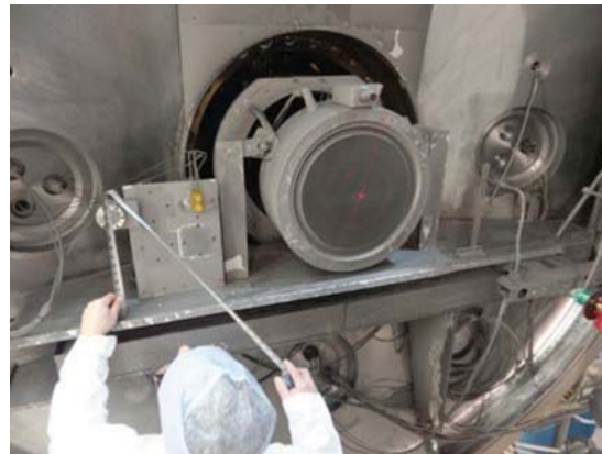
Figure 2. NEXT LDT Thruster post-test inspection
