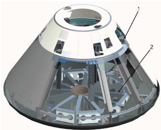
Figure 5. A Creo rendering of CM2's structural elements. Annotations: (1) LAS Attach Fittings (2) Floor Beam (1 of 12).
