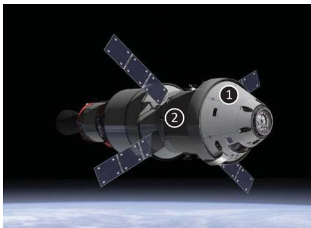
Figure 1. A rendering of the EM1 spacecraft, Orion, with annotated crew (1) and service (2) modules. Image Credit: NASA.
