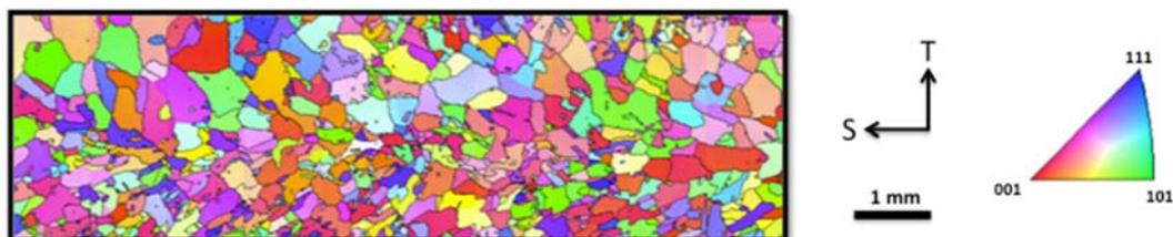
**Figure 4. L-axis inverse pole figure map in IN 718 EBF<sup>3</sup> block (HT condition).**
