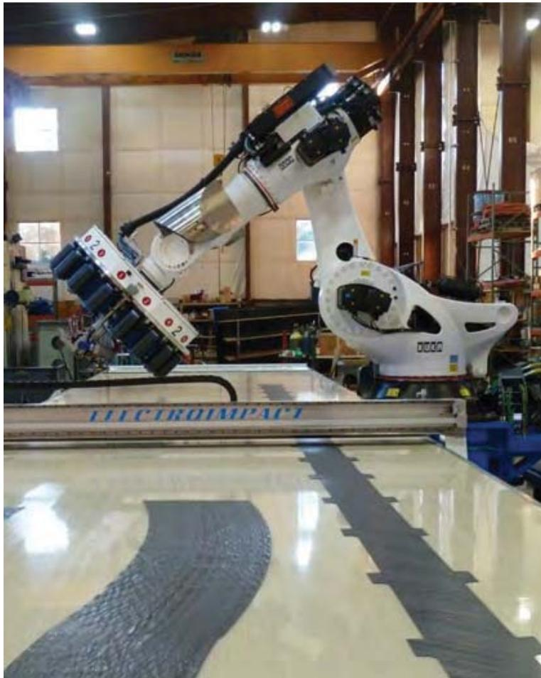
Figure 3. Robotic fiber placement system (Electroimpact).
