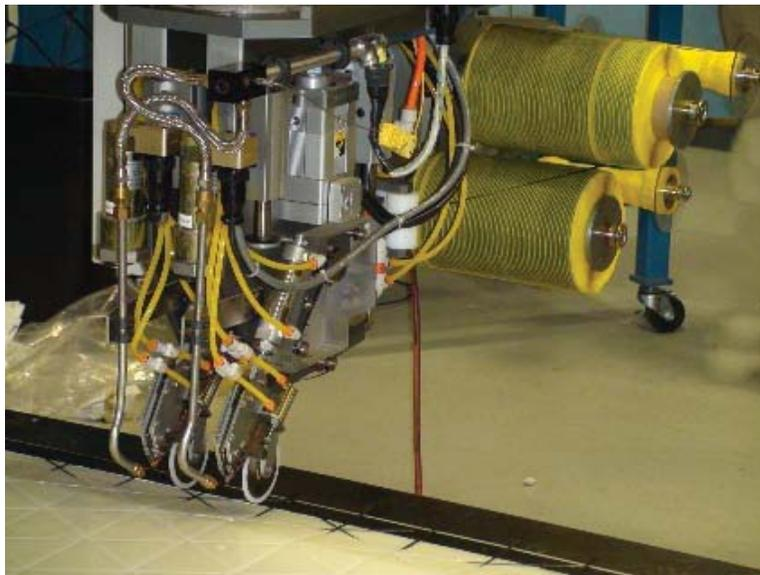
Figure 4. Composite isogrid stiffener fabrication head (ICCI).
