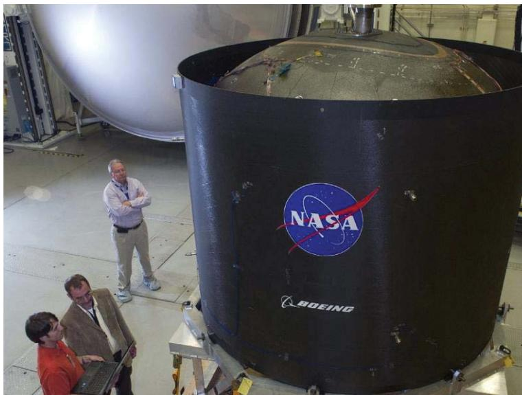
Figure 6. 2.4m-diameter composite cryotank.
