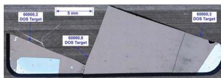
**Fig. 5:** Sample 60000 (DOS) after laser scribe cleaving.
