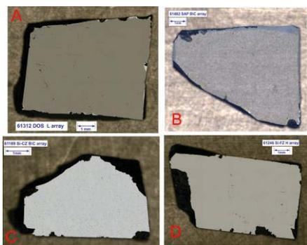
**Fig. 2:** Preview of samples that were characterized in 2014. None of the samples have been cleaned nor allocated. A) 61312 DOS L array; B) 61482 SAP B/C array; C) 61189 CZ-Si B/C array; D) 61246 FZ-Si H array
