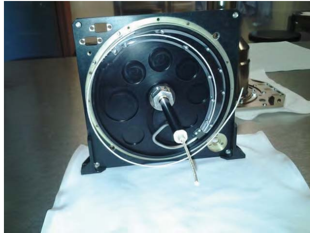
Figure 2. MMS SDP Metering Wheel Back Plate Sub-Assembly
