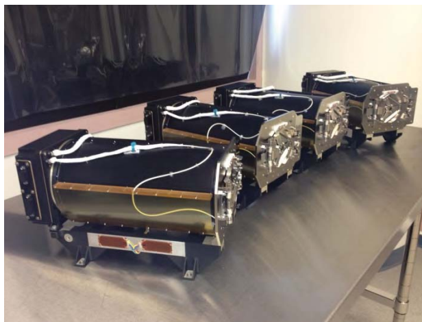
Figure 10. Flight Model MMS SDP instruments, fixed Wire Boom Termination at left
