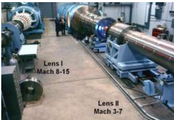
Figure 5: LENS Hypersonic Shock Tunnel
