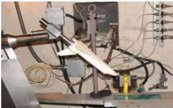
Figure 16: 0.75% Scale Ceramic Model
