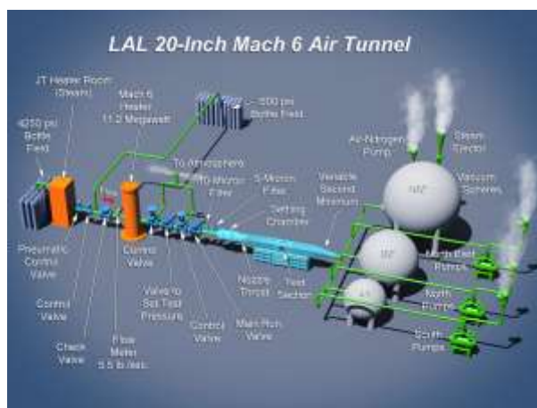
Figure 7: LaRC 20-In Mach 6 Air Tunnel
