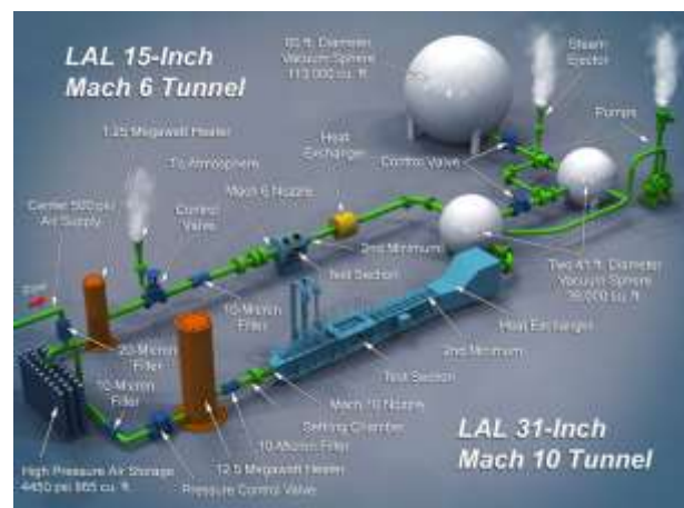
Figure 8: LaRC 31-In Mach 10 Air Tunnel
