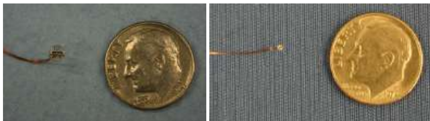
Figure 12: CUBRC Thin Film Heat Transfer Instrumentation (0.125-inch and 0.050-inch diameters)
