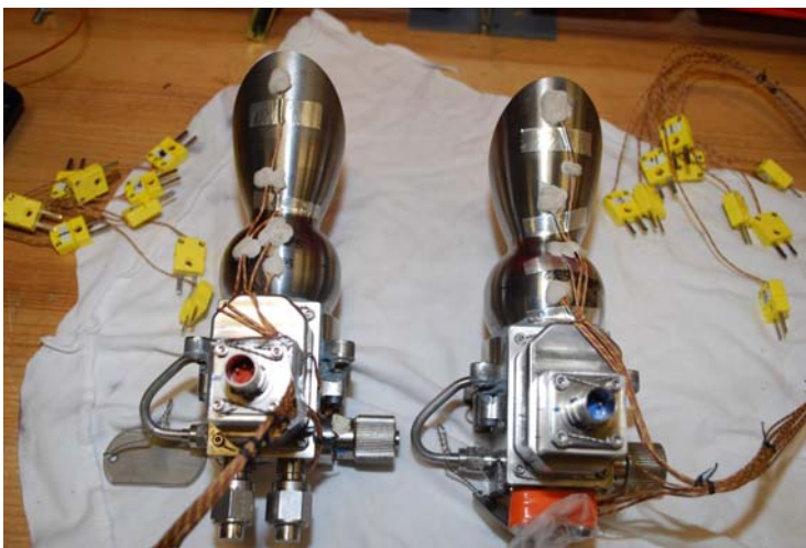
Figure 8. RS-34 Attitude Control Thruster
