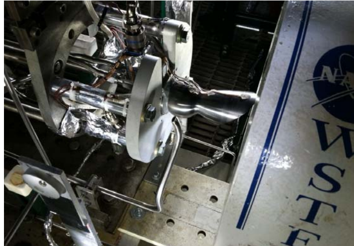
Figure 9. RS-34 Thruster Installed in TS401 at WSTF during Hot-Fire Testing
