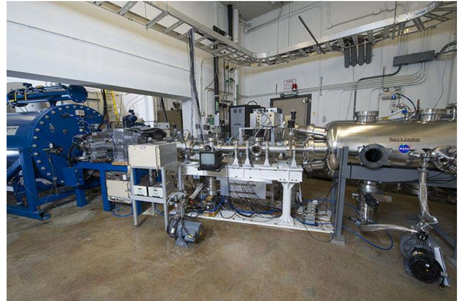
Fig. 2. The High Energy Charged Particle Radiation facility. The electron accelerator is visible on the left side (blue chamber) and the sample chamber is visible on the right side (silver chamber). The proton accelerator is not visible in this picture.
