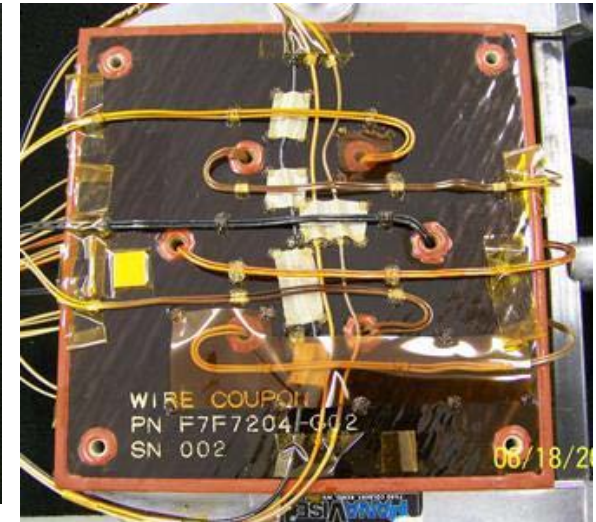
Fig. 8. Solar array wire coupon after 15 year equivalent of on-orbit UV exposure. Notice the darkening of the wire insulation compared to the BOL coupon in Fig. 7.
