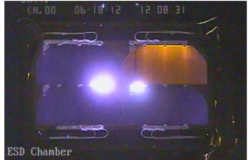
Fig. 5. ESD arc site formation on a 4-cell PV array coupon. The coupon was tested under GEO environment conditions.
