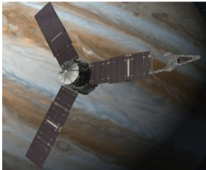
Fig. 1. The Juno probe, currently on its way to Jupiter, features the largest solar array flown by NASA on a mission other than the ISS. Image credit: NASA/JPL/Caltech.
