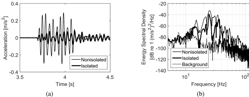
**FIGURE 2.** Sample acceleration response in the nonisolated and isolated chairs, (a) time domain and (b) frequency domain. Signals in both time and frequency domains are shown after  $w_k$  weighting for human sensitivity to full-body vibration [6].
