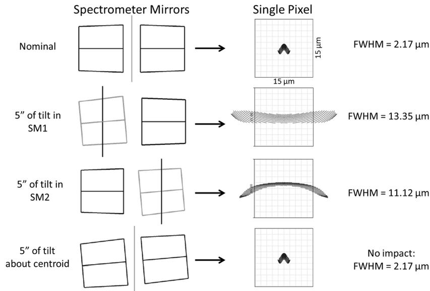
Figure 3: The spectrometer mirrors in perfect alignment produce an RMS spot radius of 0.924  $\mu\text{m}$ . Tilting SM1 by roughly 5 arcseconds produces a FWHM = 13.35  $\mu\text{m}$ . A similar case, SM2 tilted by 5 arcseconds produces a FWHM = 11.12  $\mu\text{m}$ . Both mirrors tilted 5 arcseconds about a common centroid has zero impact on performance in the detector plane.
