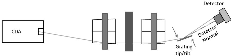
Figure 12: The grating pitch and yaw is adjusted until the reflected CDA beam pierces the center of the detector. Shims are added to offset this 0th spectral order by  $\approx 3.2^\circ$ , placing the first order at the center of the detector. Fine adjustment will be performed at the detector during X-ray calibration
