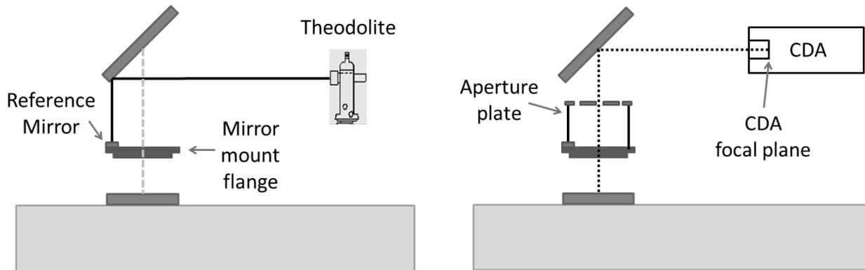
Figure 6: *Left:* The mirror mount flange is aligned using the theodolite. Tilt is removed and the axis of the flange is made parallel with the optical axis of the reference flat. *Right:* The theodolite is replaced with the CDA and an aperture plate is placed over the mounting flange. The flange is translated in the plane perpendicular to the optical axis until the CDA beam passes through the pinhole and is retro-reflected back to the CDA.
