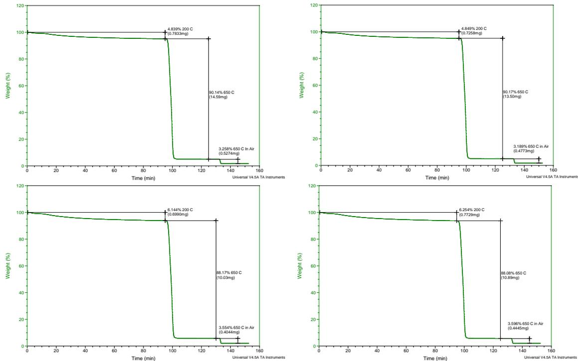
**Figure 1.** Duplicate analysis showing consistent, small increases in the low and high molar mass weight loss component of ILC Dover Armorflex® bladder material for an unirradiated control, (top), and after irradiation with 103 Gy 20-30 MeV protons (bottom) simulating a 50-year worst case exposure to solar particle event radiation.
