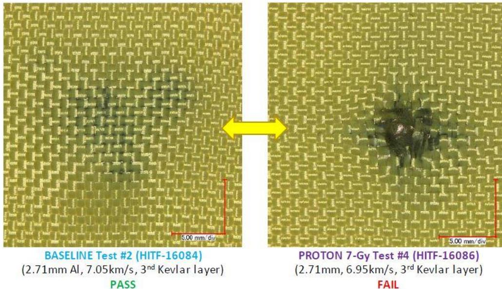
**Figure 2.** Comparison of the hypervelocity impact damage in the 3<sup>rd</sup> (final) Kevlar<sup>®</sup> layer for an unirradiated control stack (left) and a 1-GeV proton irradiated test stack (right).
