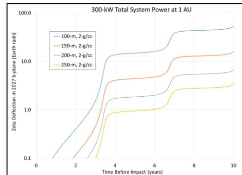
Figure 3: 300-kW System Deflection of 2017 PDC
