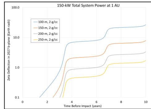
Figure 2: 150-kW System Deflection of 2017 PDC
