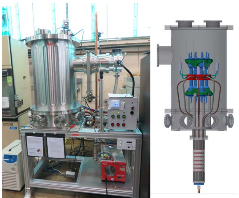
Figure 4. Photograph and CAD rendering of KRUSTY hardware inside of the vacuum chamber
