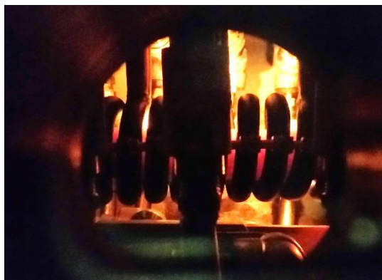
Figure 3 Fuel Element at Nominal Power
